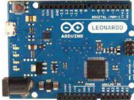
Gambar 1.2. Board Arduino Leonardo
