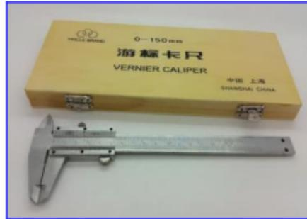
Gambar 1.2. Alat Ukur Jangka Sorong
