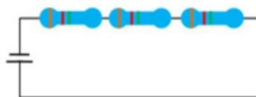
Gambar 4.3 Rangkaian seri (resistor)
