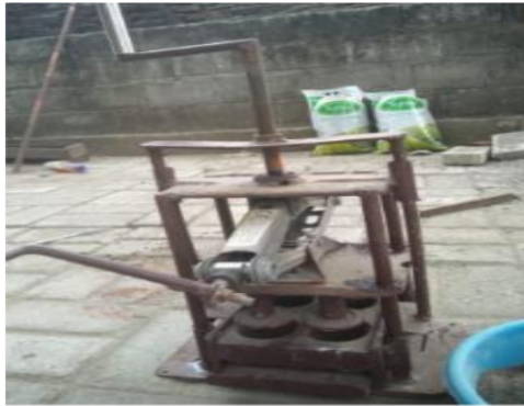
Figure 1. The ricks molding tool
