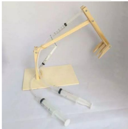
Figure 2. Simple Hydraulic Arm Instructional Aid
