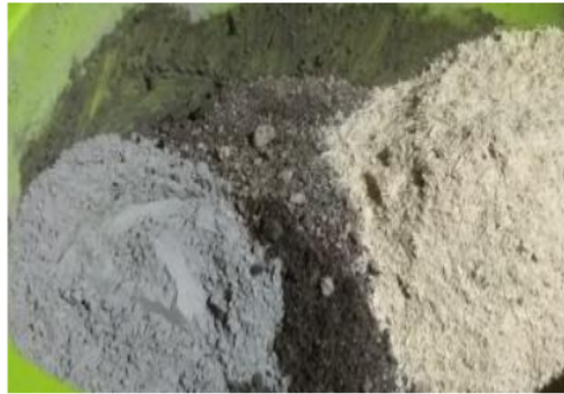
Figure 2. The corn husk powder, cement, and sand
