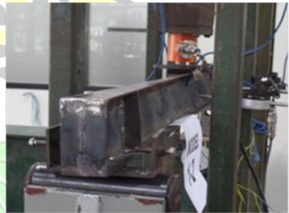
Gambar 7. Keruntuhan tekuk torsi lateral specimen
